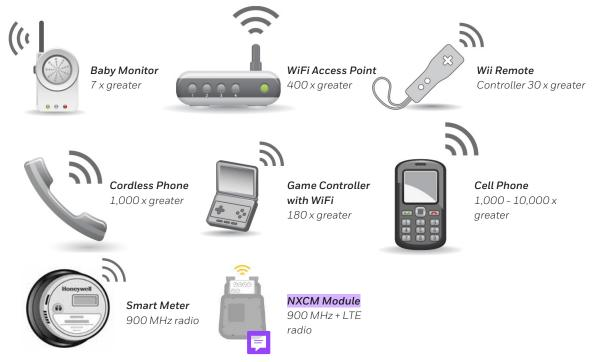
Typical values based on FCC 47CFR1.1310, which averages exposure over 30 minutes of usage. Comparative data for Honeywell Smart Meters provided by Honeywell.
